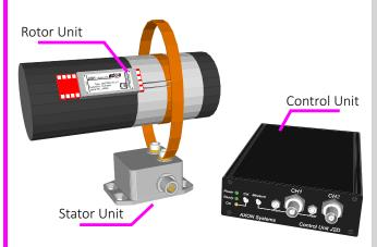
he telemetry system AXON J2D transmits the signals of two independent strain gauges. The amplified signals are made available on the Control Unit for further recording. The quality of the received digital data stream is constantly monitored, regulated and displayed via RSSI output. Thus, the telemetry system offers the possibility to simultaneously measure two strain gauge signals in the smallest space and transmit them contactless.
