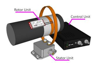
he telemetry system AXON J1DB is designed for transmitting strain gauge based measurement signals from rotating shafts under even hardest environments. During operation, a second transmission channel provides information about the inductively provided supply voltage on the rotating part of the system. The quality of the received digital data stream is also displayed via RSSI output. Through this valuable information, all important parameters for operation can be continuously monitored.
